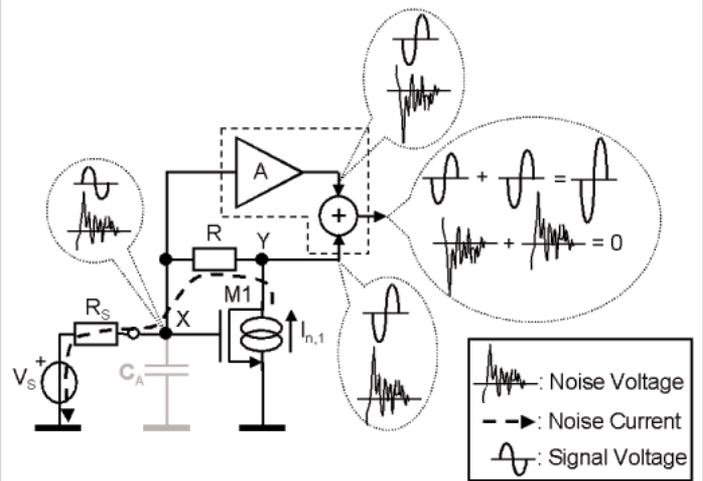
Figure 24.6.2: Noise cancelling applied to the amplifier of Figure 24.6.1c (biasing not shown).
