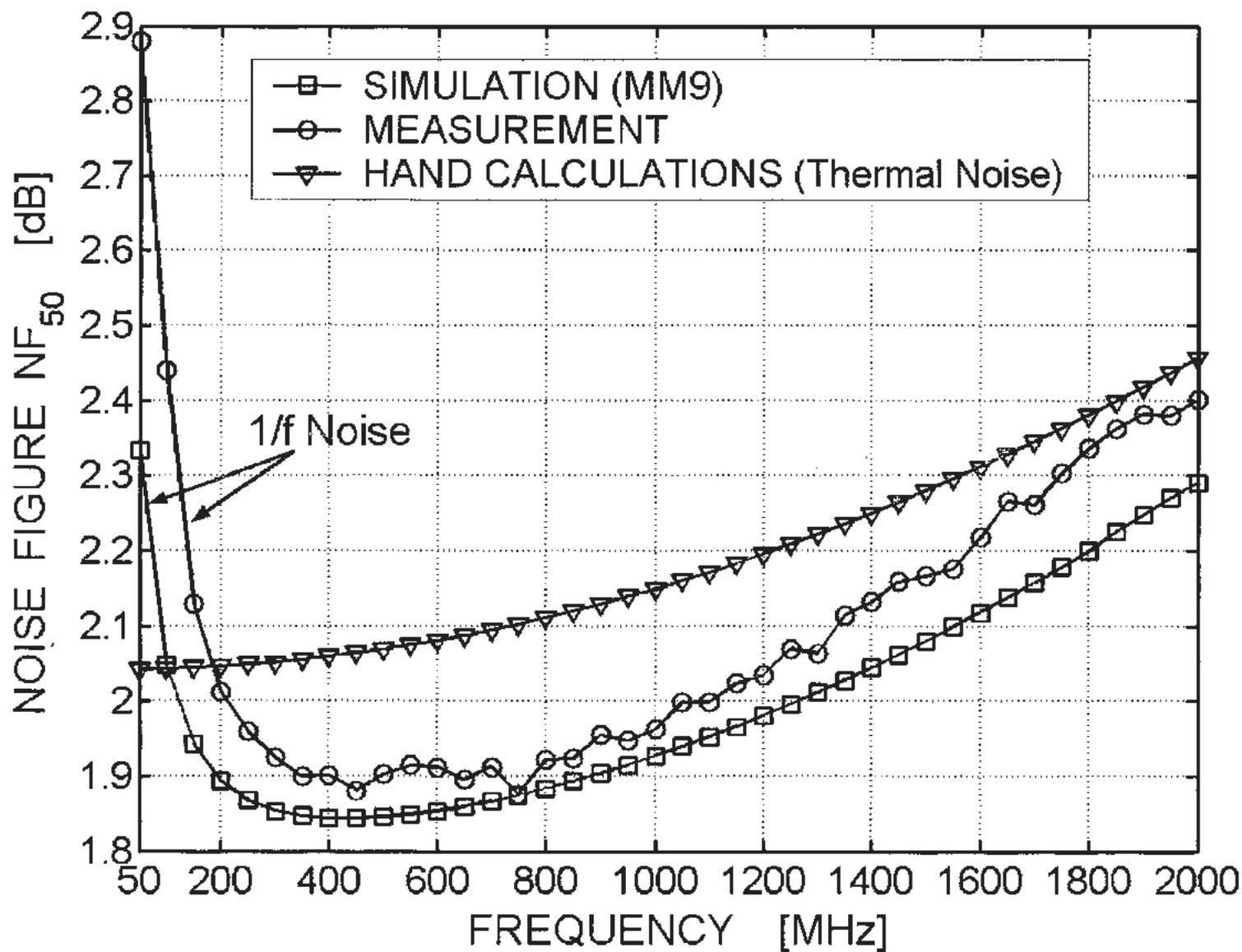
Figure 24.6.5: Measured/simulated/hand-calculated  $50\Omega$  NF.
