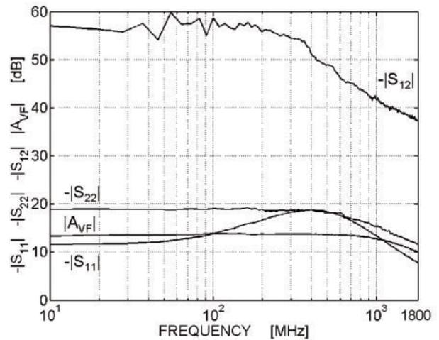
Figure 24.6.4: Measured  $S_{11}$ ,  $S_{22}$ ,  $S_{12}$  and  $A_{VF} = V_{OUT}/V_S$  ( $C_{LOAD} = C_{PAD} = 0.2pF$ ).
