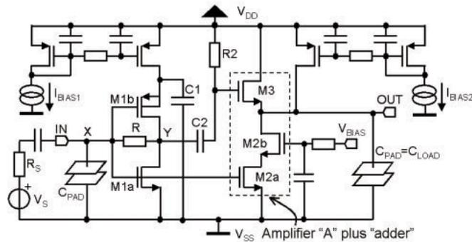
Figure 24.6.3: Schematic of the noise-cancelling wideband LNA.
