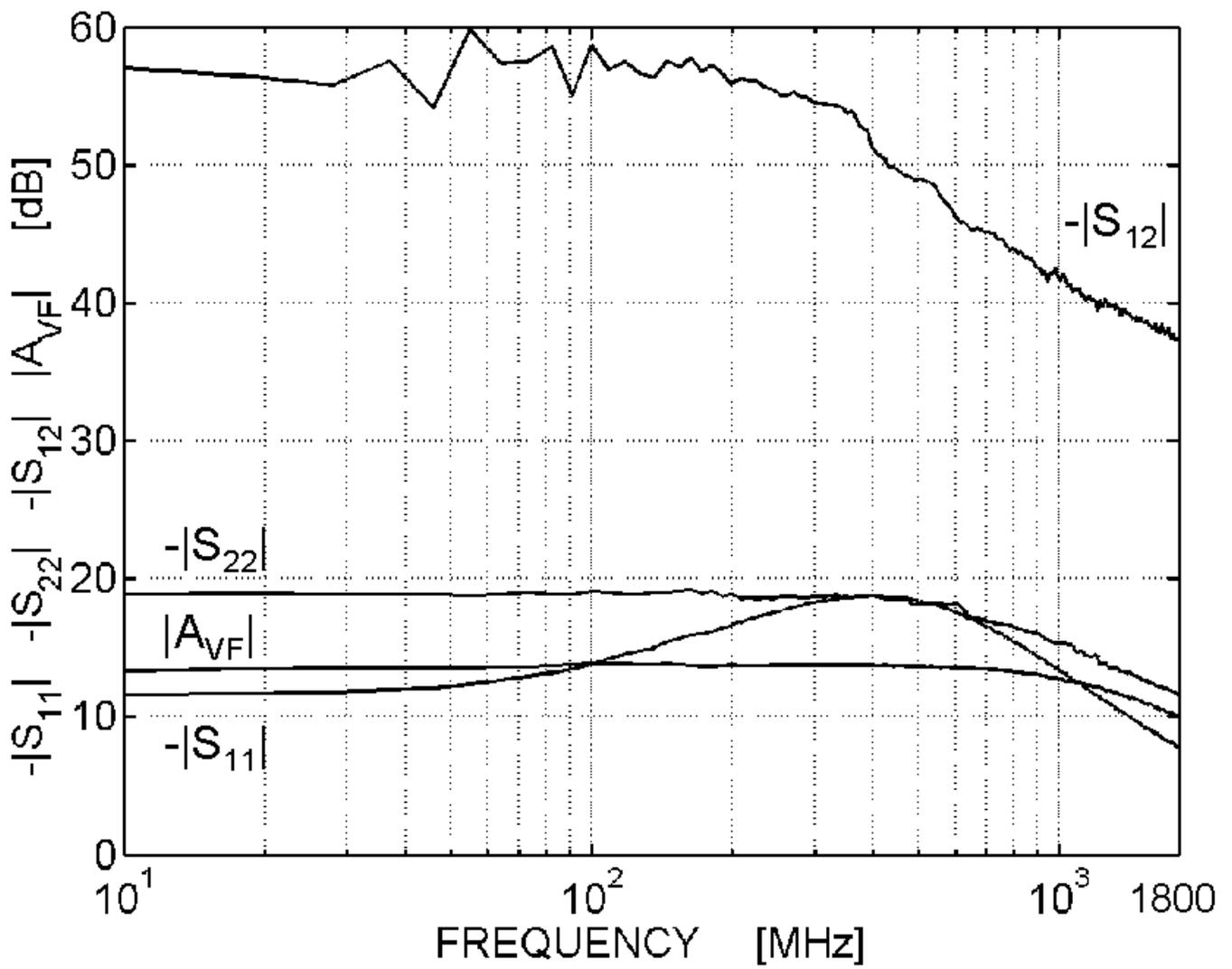
Figure 24.6.4: Measured  $S_{11}$ ,  $S_{22}$ ,  $S_{12}$  and  $A_{VF} = V_{OUT}/V_S$  ( $C_{LOAD} = C_{PAD} = 0.2\text{pF}$ ).
