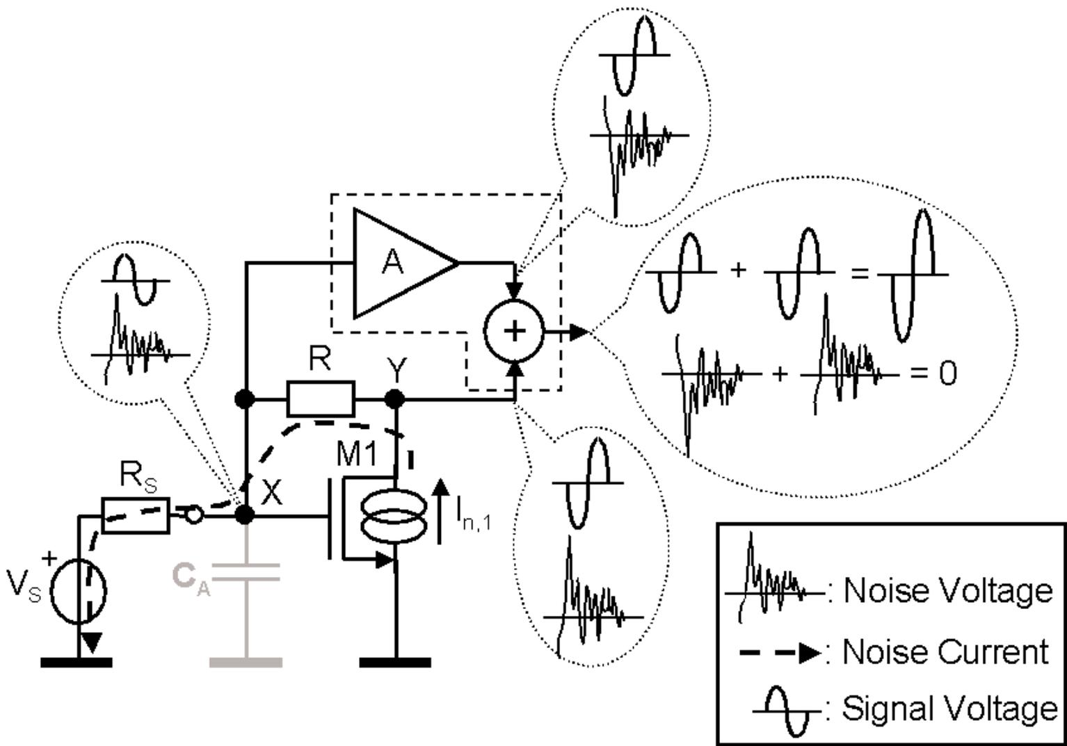
Figure 24.6.2: Noise cancelling applied to the amplifier of Figure 24.6.1c (biasing not shown).
