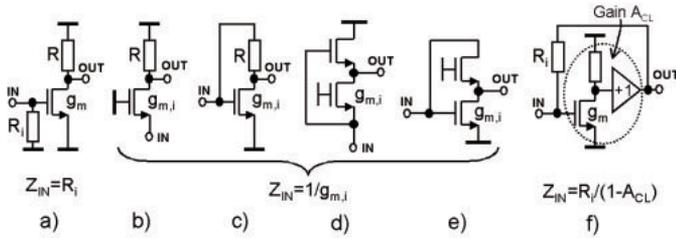
Figure 24.6.1: Common wideband CMOS LNAs (biasing not shown).
