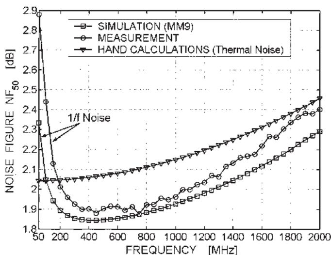
Figure 24.6.5: Measured/simulated/hand-calculated 50Ω NF.
