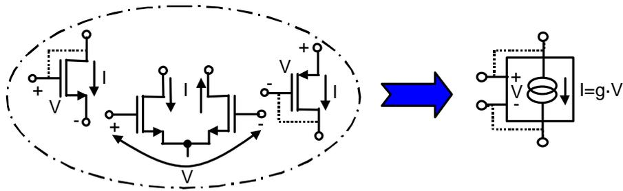
Fig.1: VCCS representation of simple MOS circuits.
