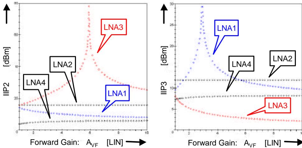
Fig.7: IIP2<sub>dBm</sub> and IIP3<sub>dBm</sub> versus the forward gain  $A_{VF,V}$  upon  $\min P_{LNA,min}$ .
