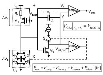
Figure 19.5.4: Actual implementation of a switched-capacitor relaxation oscillator.
