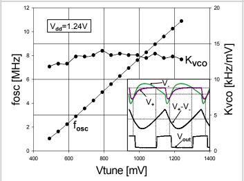
Figure 19.5.5: Measured waveforms, frequency tuning range and frequency tuning gain (Agilent DSO6104A oscilloscope and LeCroy AP033 active differential probe, R&S FSP spectrum analyzer).
