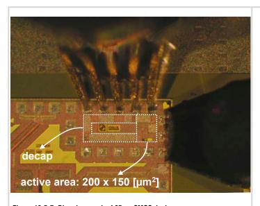
Figure 19.5.7: Die micrograph of 65nm CMOS design.
