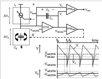
Figure 19.5.2: Block-level schematic of a switched-capacitor relaxation oscillator
