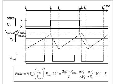
Figure 19.5.3: Technique to filter out the noise of the oscillator comparator (cmp  $_{\! \text{osc}}).$
