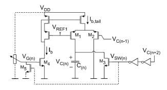
Fig.2: Circuit schematic of section (n) of the coupled sawtooth ring oscillator.
