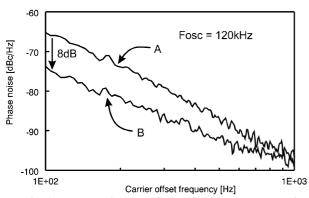
Fig.6: Phase noise [dBc/Hz] of the sawtooth oscillator as a function of carrier offset frequency for the constant bias (curve A) and switched bias condition (curve B): 8 dB reduction is achieved at 100 Hz.
