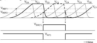
Fig.3: The capacitor voltages of the 6-stage coupled sawtooth oscillator and signals Vsw(1) and VG(1) that are used in stage 1 (see fig. 2 with n=1) to respectively discharge C1 and accomplish switched biasing.
