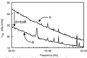
Fig.5: Measured baseband spectra for constant bias (curve A) and switched bias (curve B:  $f_{\text{switch}} = 100 \text{kHz}$ , duty-cycle = 50%).
