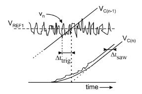
Fig.4: The effective filtering of noise  $v_n$  on the threshold level  $V_{REFI}$  in the coupled sawtooth oscillator results in a smaller time error  $\Delta t_{saw}$  compared to the time error  $\Delta t_{trig}$  that would appear in a regenerative oscillator.
