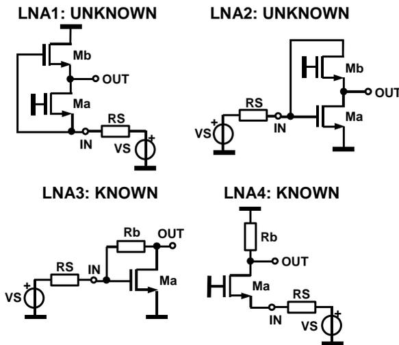
**Figure 6:** Simplest implementations of the graphs of Figure 5 based on Figure 4 (biasing not shown (voltage bias sources replaced by short-cut to ground, current source by open)).
