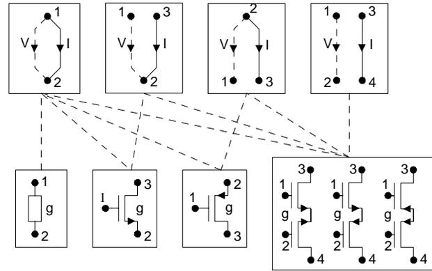
**Figure 4:** The interconnections between the V- and I-branches, and their relative orientation determine the possibilities to implement a VCCS.
