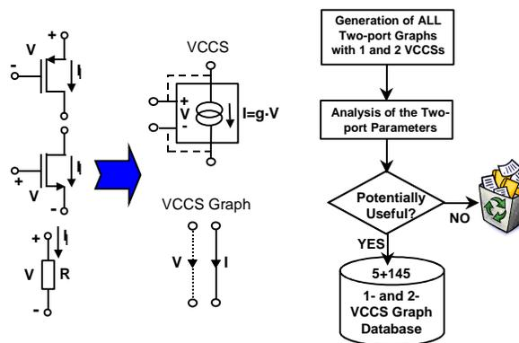
**Figure 1:** Components in Transconductance based circuits functionally behave as a Voltage Controlled Current Source (VCCS). Its graph representation is a V- and I-branch. All linear graphs of two-ports with 1 and 2 VCCSs have been generated. Potentially useful ones are stored in a VCCS Graph Database.
