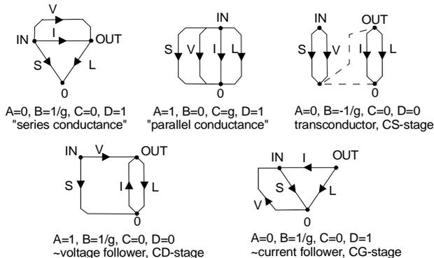
**Figure 3:** All potentially useful graphs of circuits with a source (S), load (L) and one VCCS (V and I) (see text).
