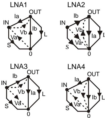
**Figure 5:** Graphs selected from the VCCS graphs database based on LNA functional requirements.
