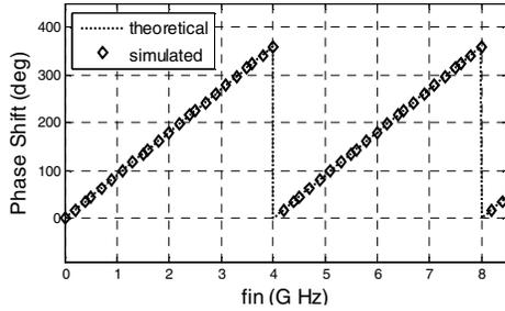
Figure 4. Phase shift with synchronized output ( $f_s=1\text{GHz}$ , and  $\Delta t=250\text{ps}$ )
