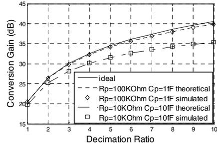
Figure 6. Conversion gain of RF charge sampler at 2.4GHz
