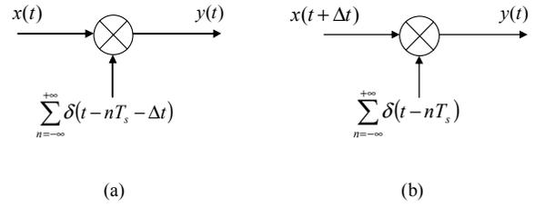
Figure 3. Two equivalent general models for delayed sampling: (a) delayed sampling impulses; (b) delayed input signal.
