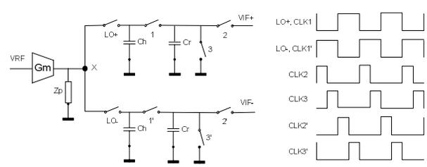
Figure 5. An RF charge sampler with an example of clock scheme
